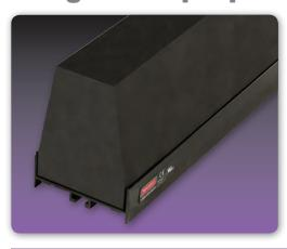
**SE-45 & SE-75 Sensing Bumpers** are designed for general-purpose, heavy-duty applications. When deformed by contact or impact, they provide a signal in the form of an electrical contact closure. At the same time, the large, compliant surface and substantial overtravel cushioning helps protect personnel and equipment from injury or damage. Operating force is 20 pounds nominal.
