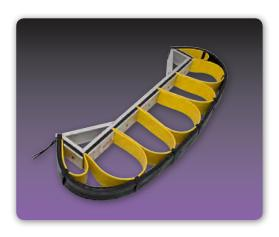
The VBL-Series High-Impact Sensing Bumpers are designed to survive repeated crushing impacts that would destroy conventional bumpers. When deformed by contact or impact, they provide a signal in the form of an electrical contact closure. They are suitable for use on AGVs, mobile platforms, traveling conveyors, and other moving equipment or machinery. Sensitivity is uniform over the entire bumper surface, including any curved areas.
