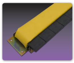
**SE-C Custom Sensing Bumpers** are designed to fit specific application needs. When deformed by contact or impact, they provide a signal in the form of an electrical contact closure. They have a large, compliant surface that helps protect personnel and equipment from injury or damage. The nylon-reinforced exterior housings are resistant to water, oil, hydraulic fluids, and coolants. Mounting options include studs and threaded holes.
